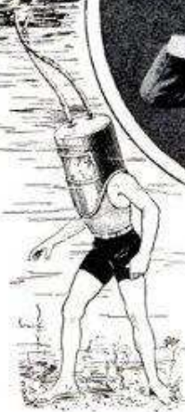
Completed water-heater diving helmet.
