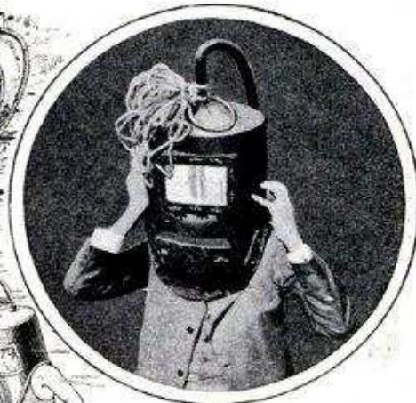
Completed water-heater diving helmet.
